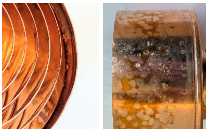
Figure 46: On this capacitor specimen, arcing marks are clearly visible.
