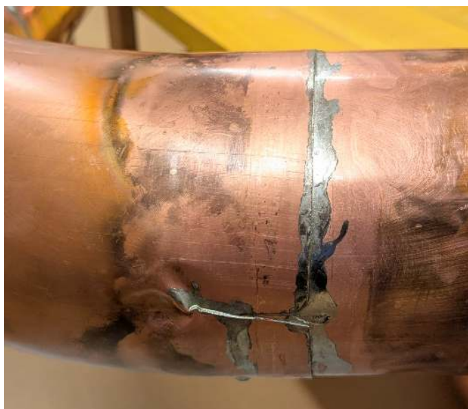
Figure 27: Soldering joint after removing flux residues.
