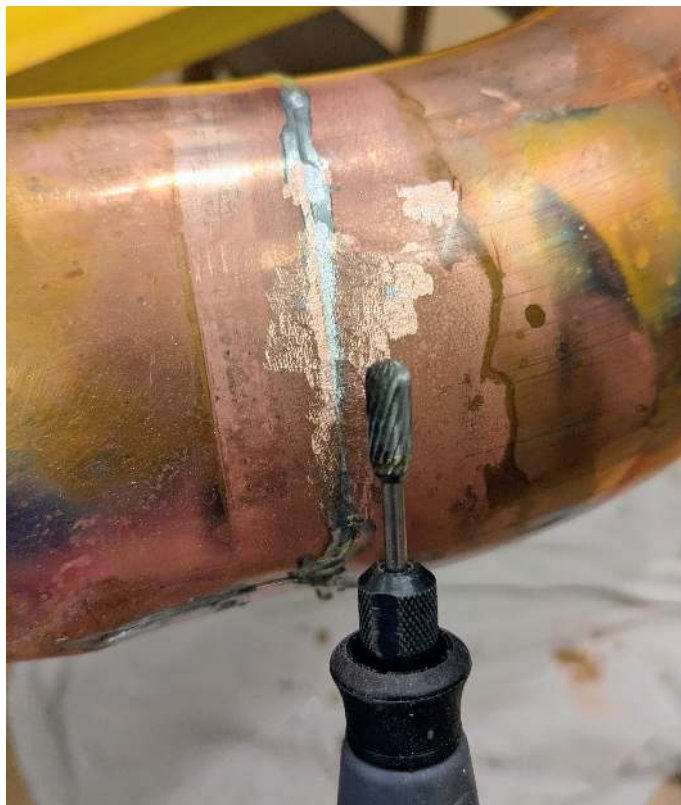
Figure 28: Removing excess solder with a milling cutter.
