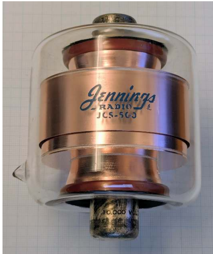
Figure 51: Jennings JCS-500-10S vacuum capacitor. Two of these are used.
