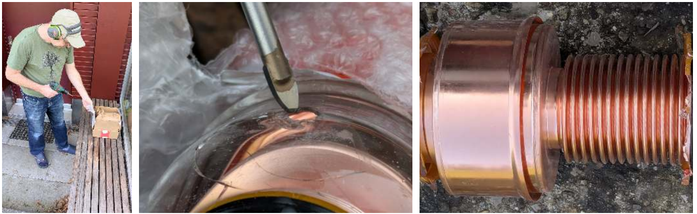
Figure 38: Left: the author and the capacitor wrapped in cardboard as implosion protection. I had no idea whether opening it would be dangerous — it took some courage to drill into the glass envelope. The sound was just a soft blob, not loud at all. Center: glass drill bit; the vacuum is gone. Right: the glass is then removed with a hammer, revealing the beautifully colored copper inside.
