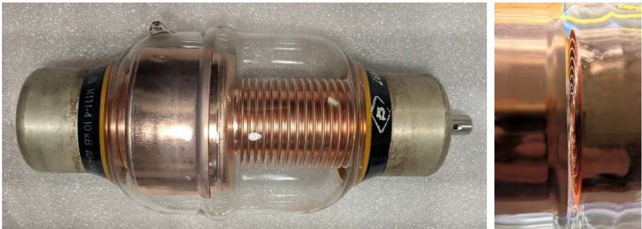
Figure 37: Left: variable vacuum capacitor KP1-4 10–500 pF. Right: when the capacitor is set to minimum capacitance, the concentric copper tubes are visible.
