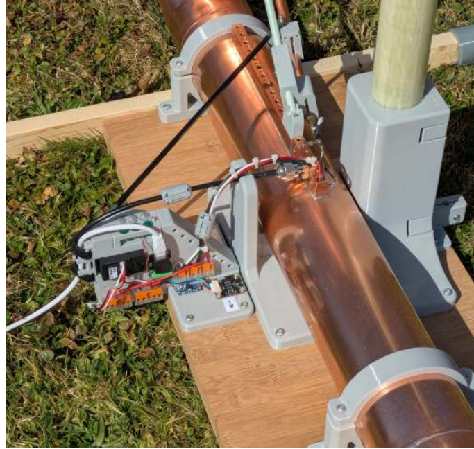
Figure 66: Cable routing and placement of the electronic components are exactly in the symmetry plane of the antenna. Left, black: servo_z for coupling adjustment; below: magnetometer for azimuth control. Not shown in the image: servo_h for azimuth control.
