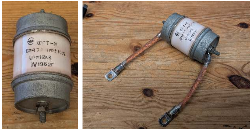
Figure 53: Markings: type designation \Phi\Gamma\Gamma-\text{И} (FGT-I series, PTFE dielectric), 4700 \text{ пФ} \pm 10\% ( 4700 \text{ pF} \pm 10\% ), U_p = 12 \text{ кВ} (peak voltage 12 kV), IV 1962 r (4th quarter 1962). Translation without guarantee.
