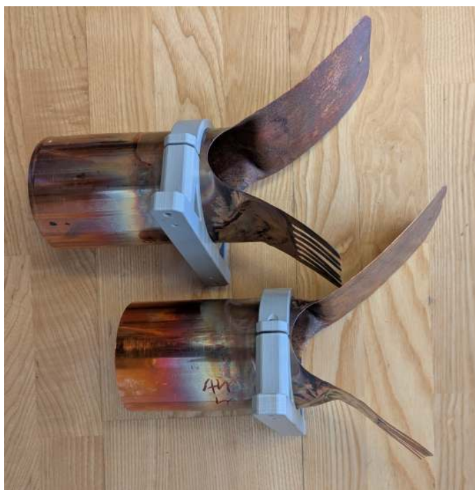
Figure 25: Annealed and bent transitions. The surface is still black from copper oxide.
