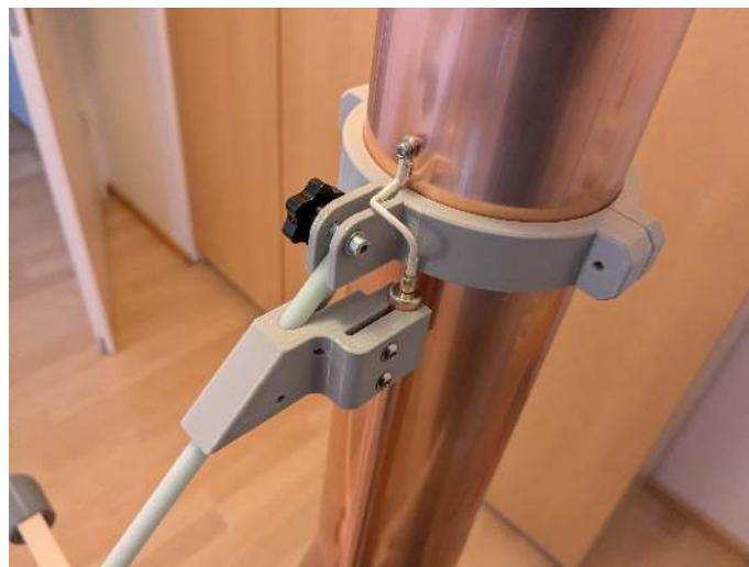
Figure 64: Pivot joint in the center of the loop with galvanic connection to the main loop.
