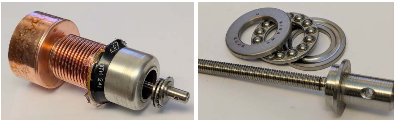
Figure 39: Turning the shaft clockwise retracts one set of vanes, reducing the capacitance. An internal spring (not visible in the photo) pushes the copper bellows back to full extension when the capacitance is increased.
