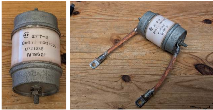
Figure 52: Markings: type designation \Phi\Gamma\Gamma-\text{И} (FGT-I series, PTFE dielectric), 4700 \text{ пФ} \pm 10\% ( 4700 \text{ pF} \pm 10\% ), U_p = 12 \text{ кВ} (peak voltage 12 kV), IV 1962 r (4th quarter 1962). Translation without guarantee.
