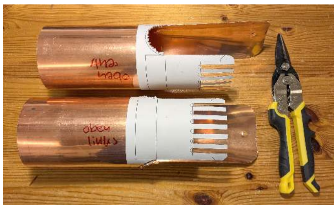
Figure 23: Transitions from pipe to capacitors with glued-on cutting patterns.
