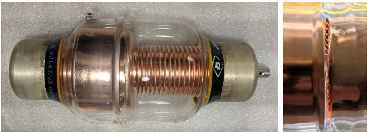
Figure 36: Left: variable vacuum capacitor KP1-4 10–500 pF. Right: when the capacitor is set to minimum capacitance, the concentric copper tubes are visible.
