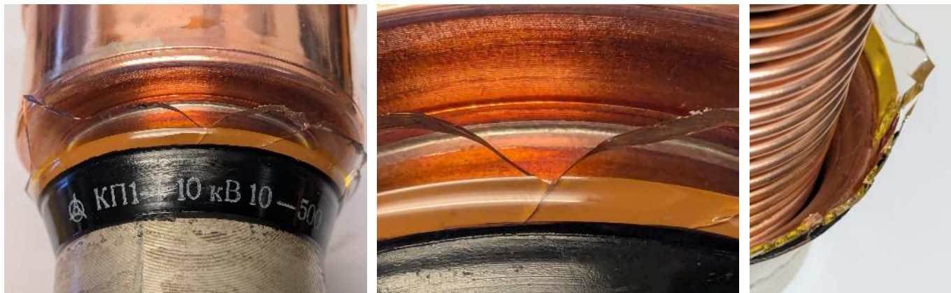
Figure 43: The transition from glass to copper was made by fusing glass and copper together.
