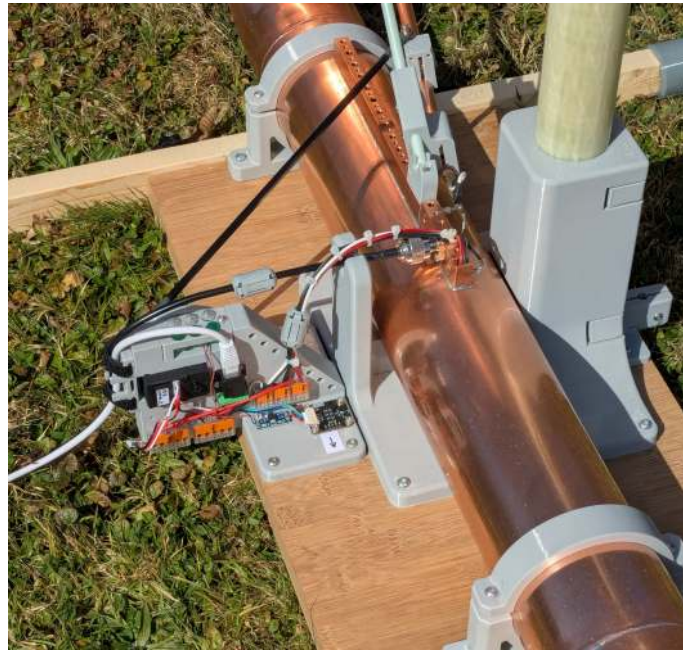
Figure 65: Cable routing and placement of the electronic components are exactly in the symmetry plane of the antenna. Left, black: servo_z for coupling adjustment; below: magnetometer for azimuth control. Not shown in the image: servo_h for azimuth control.
