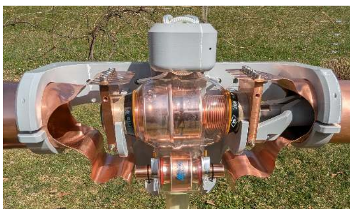
Figure 33: Configuration for 10 m to 40 m: only the variable capacitor is connected. Capacitor A is mechanically mounted, but the side screws are not inserted. The gap between the copper tabs and the capacitor end caps is about 10 mm.
