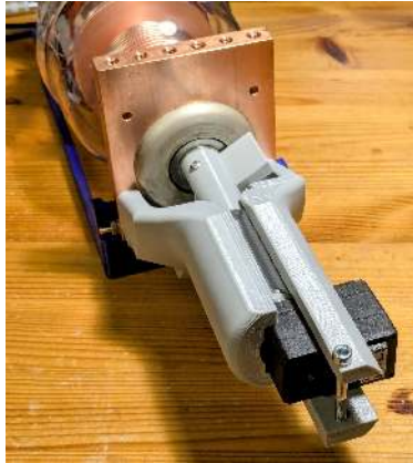
Figure 49: Capacitor assembly. The servo_f is located inside the copper tube and is therefore in a field-free region.
