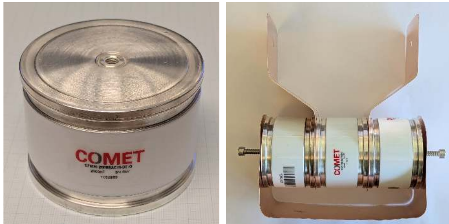
Figure 57: Left: a single capacitor with 2800 pF. Right: capacitors loosely connected with metal sheets to illustrate the wiring.
