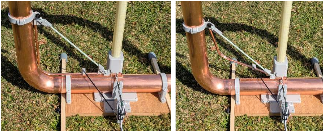
Figure 63: Left: small coupling; right: large coupling. The servo_z automatically adjusts the coupling and is connected via a black fiberglass rod (not carbon fiber, which would be electrically conductive).
