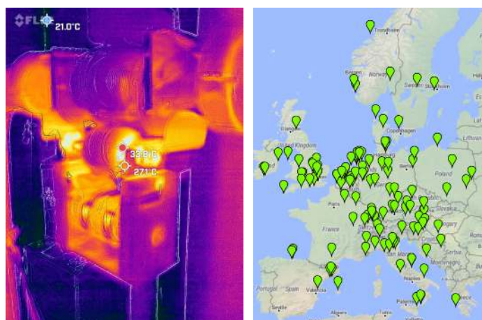
Figure 61: Left: after 10 minutes of transmitting at 100 W, the Comet capacitors heated up by 3.7 °C, the Jennings capacitor in the center by 0.3 °C, and the metal sheet connecting to the Jennings capacitors by 8 °C. Right: during a test on April 10, 2026, FT8 signals were decoded within a radius of approximately 1500 km. This is quite remarkable considering that the radiated power is at most 70 mW. Source: pskreporter.info.
