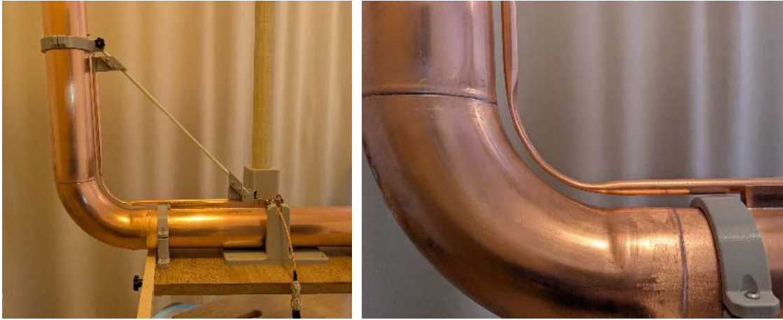
Figure 62: Gamma match constructed from 12 mm diameter copper tubing with a total length of 0.7 m.
